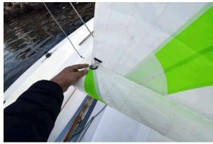
13. While rolling the sail, have the crew gently lower the mainsail using the main halyard. The crew should also assist the roll on the luff side of the sail.
