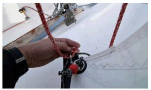
11. Release the outhaul and remove the ball stopper knot from the clew.
