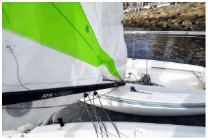
9. Release the main halyard from both the horn cleat and the jam cleat. Then slowly lower the mainsail. Do not let the boom drop and slam into the boat. Unhook the reefing cringle ring from the hook on the boom.
