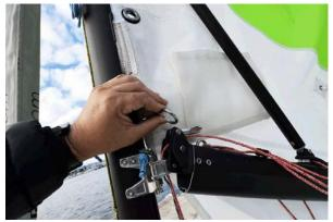
10. Remove the figure 8 knot from the end of the reefing line.
