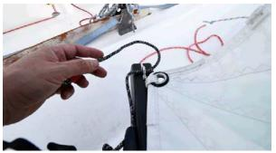
12. Slide the clew slug out of the track. Then roll the sail upwards keeping the leech side of the sail flush.
