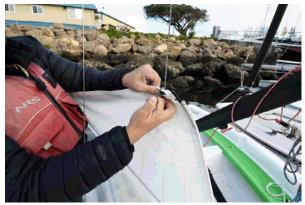
15. Secure the main halyard to the boom using a ball on a bight knot through the outhaul fairlead.
