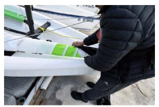
18. Cleat the mainsheet to prevent the boom from swinging, and coil it neatly over the mainsheet block. Coil up any other loose lines.
