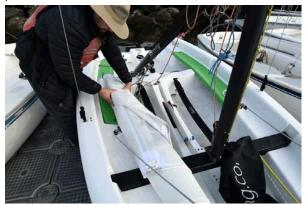
17. Place the mainsail into the sail bag luff side first. This way the next time you rig the boat you should place the sail with the open end towards the stern. This will ensure that the sail does not need to be flipped to be raised.
